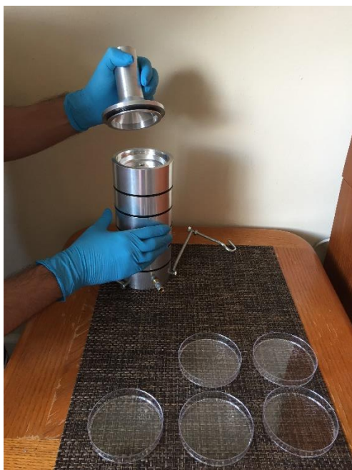
Figure 4.2.a. Disassembling the inertial cascade impactor to retrieve samples.
