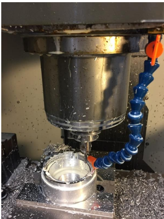
Figure 3.9. Manufacturing base on CNC milling machine
