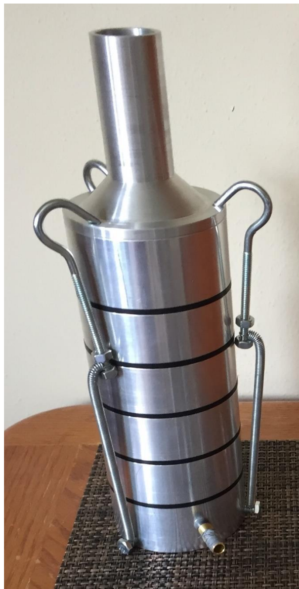
Figure 3.13. Fully assembled Inertial cascade impactor
